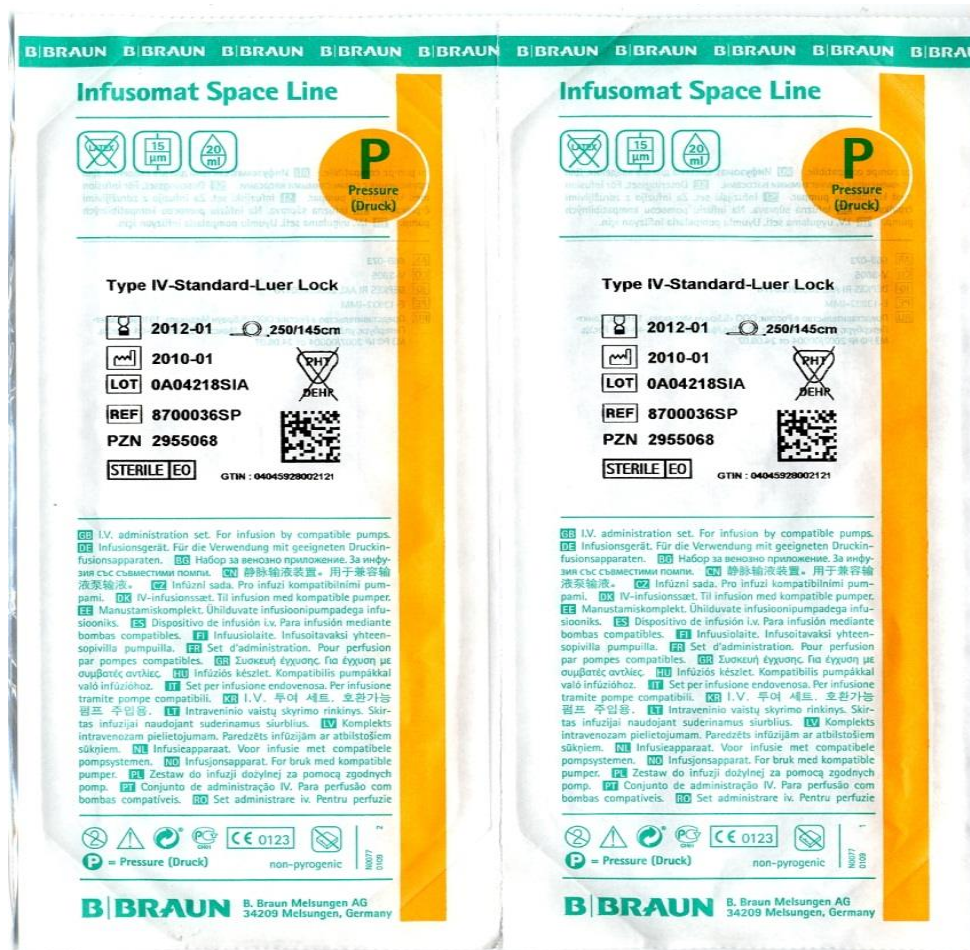
Figure 3: Example of a label with a UDI, on primary packaging. This is the final layer of packaging, which is in direct contact with the product itself. The unique product number, lot number and expiry date are indicated both in script and in a Data Matrix on the label:
